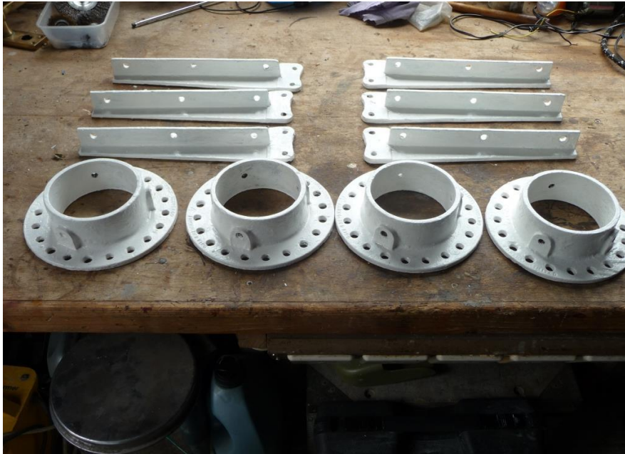
Figure 6 Renovated Collars and Bracket Arms
