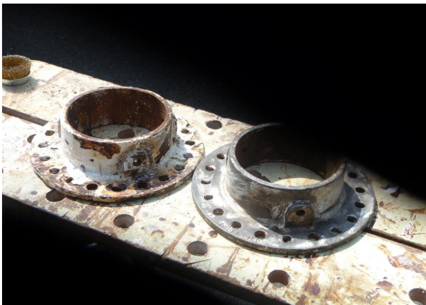
Figure 5 Collar Before and After Cleaning
