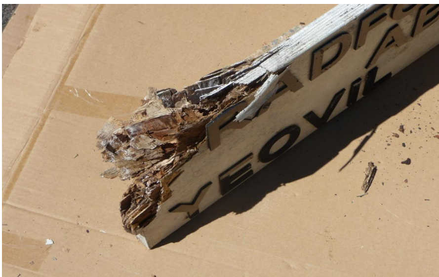
Figure 7 What Happens to DCC Highways Plywood Arm Fingers
